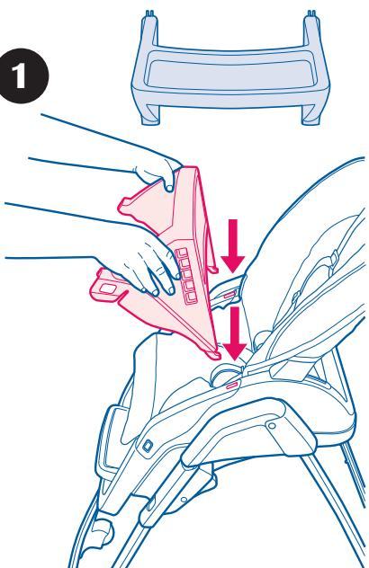
Insert hooks on the back of snack tray into receiving slots.
